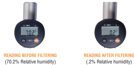
Compare the humidity reading before and after filtering with DeVilbiss DAD-500
